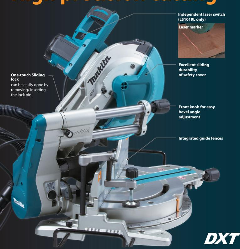
Diameter of slide pipe is changed from 25mm to 30mm. Moreover, by redesigning Arm section shape, the precision at bevel cutting is increased.
