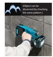
For detecting composite objects, such as rebars and cavities, in concrete block or brick wall
