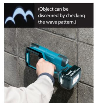
For detecting composite objects, such as rebars and cavities, in concrete block or brick wall
