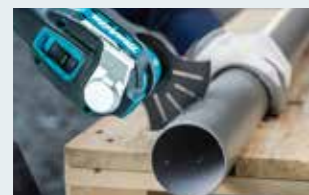
Cutting PVC, FRP pipes
