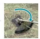
Reverse switch for clearing entangled weeds and grass from cutting head
